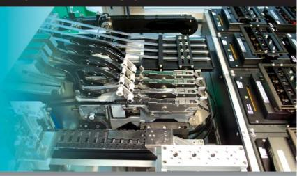
The latest H9800 programmers and N-type socket boards incorporate new buffer designs, allowing 4 Memory devices to be serialized, or 4 NAND Flash to be programmed, simultaneously at each cycle.
